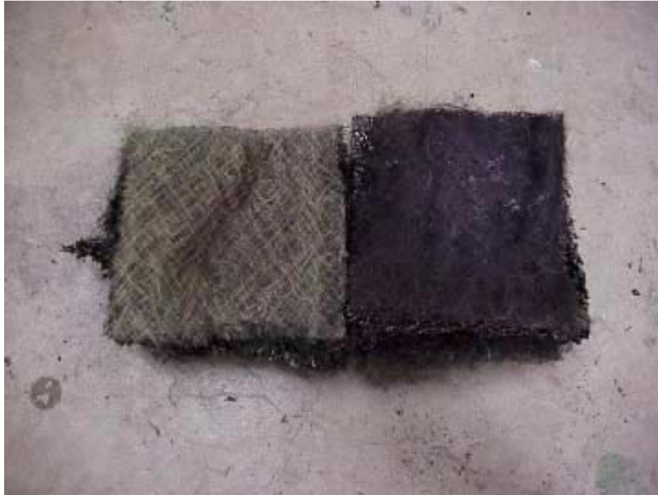
Figure 10 - Paint loaded filter after test (sub-critical).
